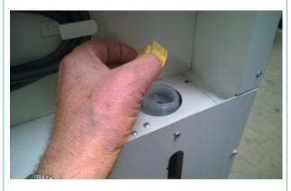
The water levels in the room unit will be correct when delivered. However if for some reason the water level has fallen, top up as required.
