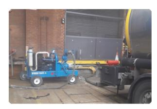
Performance Max head: - 98 m, Max flow: - 44 l/s Weight 1004 kg with fuel / 907 kg without fuel Dimensions 940 x 1450 x 1530 MM Noise level @ 7m = 77 - 82 dBAFuel capacity 122 litres Pipe connections Suction: - 4" Table D or 4" Bauer Discharge: - 2 1/2" Instantaneous adapter or (3" Bsp) Fuel Consumption Full load @ 2800 rpm:-10.8 litres/hour
