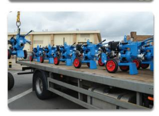
Performance Max head: 28 m, Max flow: 15 l/s, Max solid: 28 mm
