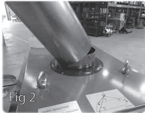
Fig 2 : Remove protective cover and fit 1mt exhaust flue.
