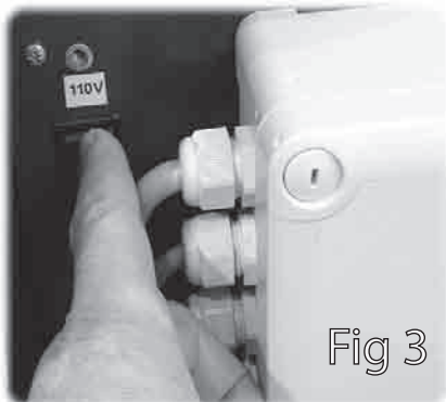
Fig 3 Set rocker switch to required voltage.
