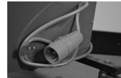
Fig 3 Connect to selected electrical supply and ensure cable is fully unwound from storage bracket
