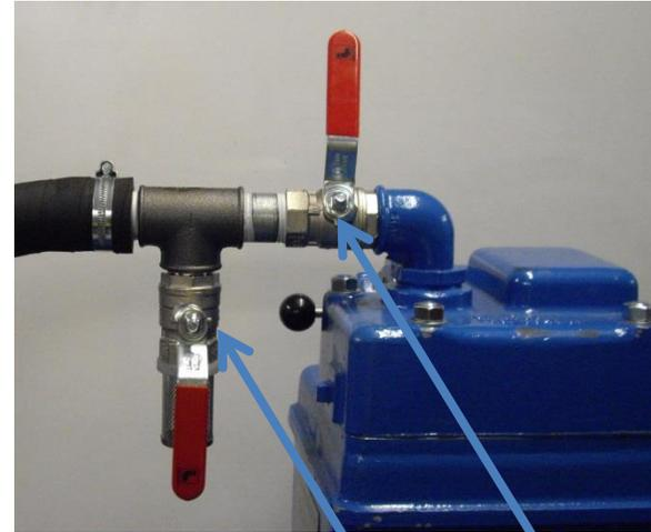
VACUUM SHUT OFF VALVE CLOSED
