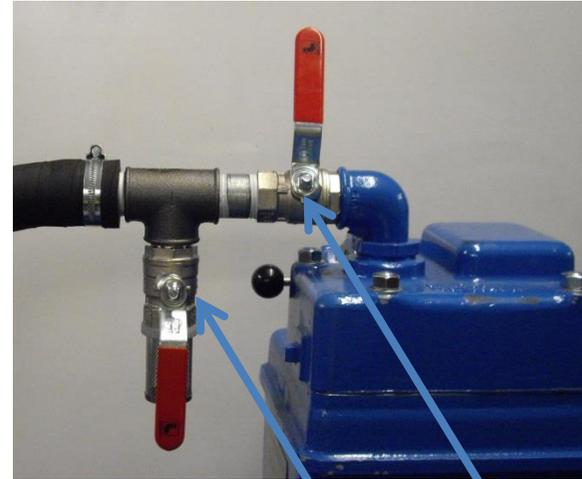
VACUUM SHUT OFF VALVE CLOSED
