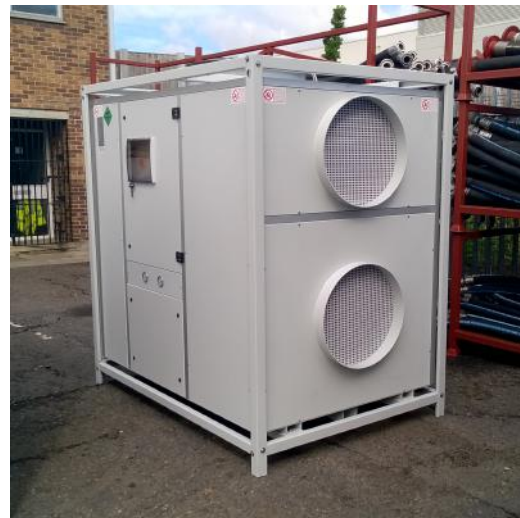
Fig 5: Normal running conditions will have the outlet Air temperature displayed on the controller and the condensing fan motors on top of unit will only run when the unit needs to remove the heat from the condensing coil
