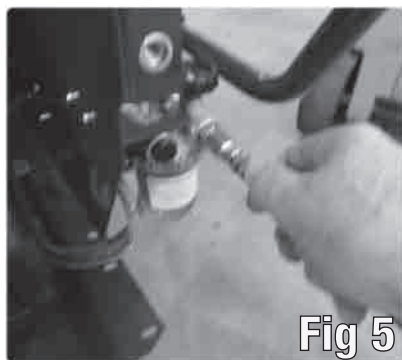
Fig 5 : Connect fuel supply line
