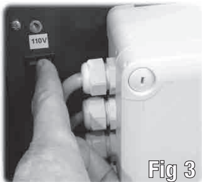
Fig 3 : Set rocker switch to required voltage.
