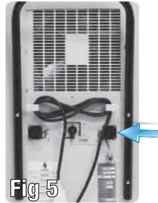
Fig 5 : The condensate pump is close coupled electrically to the machine via a built in auxiliary connection. Up to 20 metres of flexible drain hose can then be routed to a suitable drain point.
